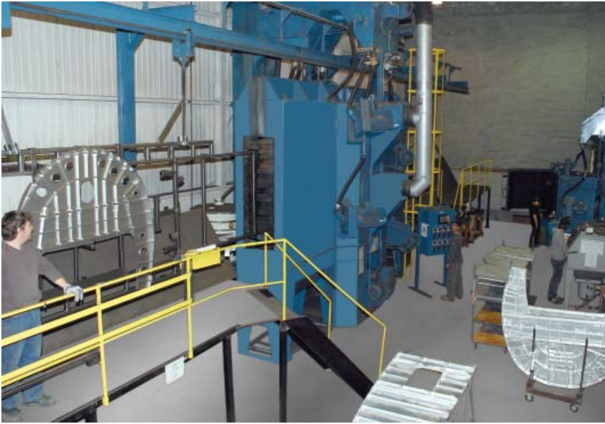
Large component shot peening and peen forming capability
