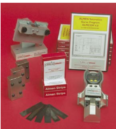
Peening Accessories GmbH donated Almen gages, strips and holders and software for the Almen saturation curve
